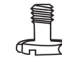
2x Screw (1/4-20UNC) for mounting the HTC Vive tracker on the adapter
